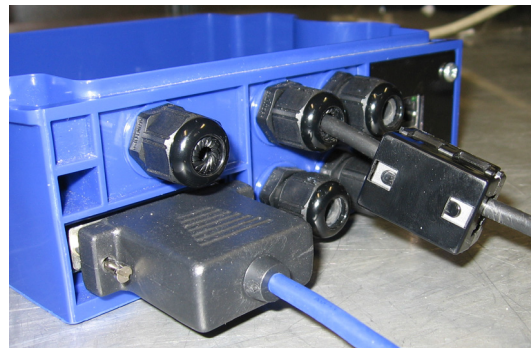
Figure 5 - Ferrite Installation Example
