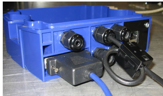
Figure 6 - Ferrite Installation Example
