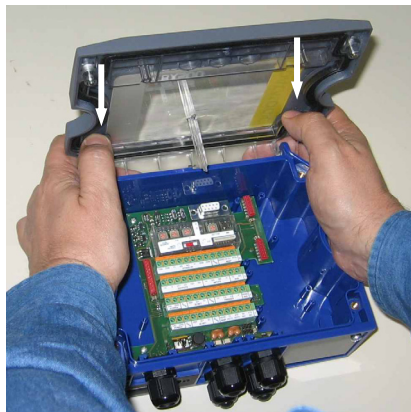
Figure 2 - Removing CBX500 Cover
